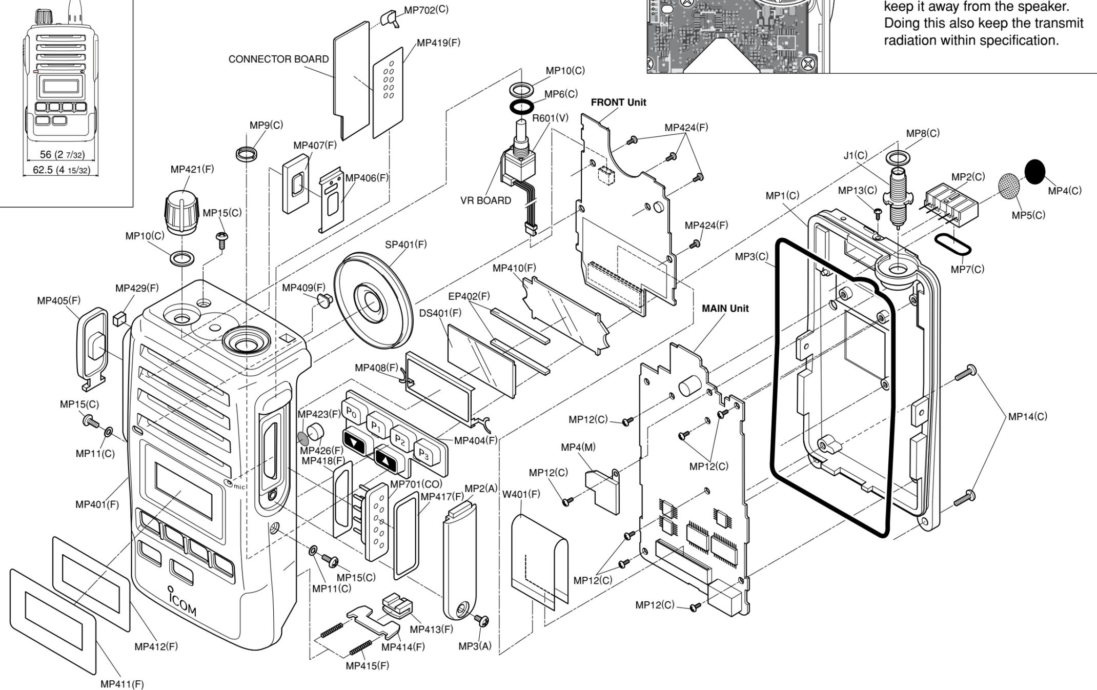
**UNIT abbreviation** (C): CHASSIS PARTS, (M): MAIN UNIT, (CO): CONNECTOR BOARD, (V): VR BOARD, (A): ACCESSORIES, (F): FRONT UNIT
